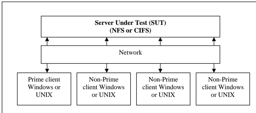
The minimal configuration consists of one load generating client, and one NFS or CIFS server. The server is often referred to as the SUT (Server Under Test) in the documentation below.
